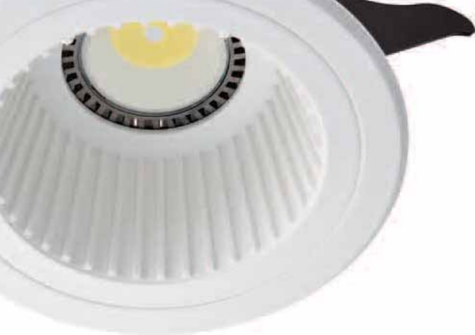
MR16 Corrugated Pattern Power Consumption - 3W Dimensions - Ø120xH90mm Hole Size - Ø105mm CCT - 3000K / 6000K Replacement - Halogen 24W Input - AC100-240V 50-60Hz
