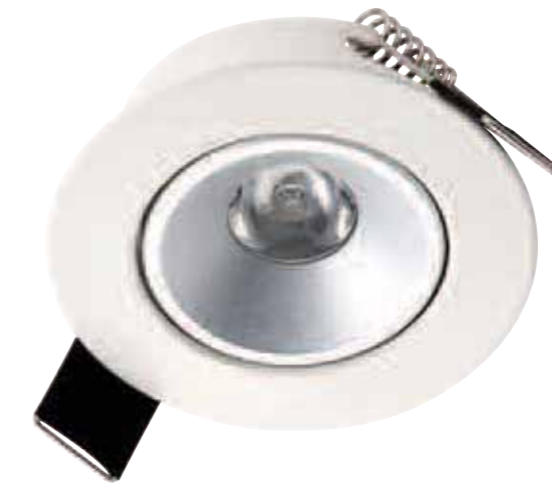
MR8 Size Accent Downlight Power Consumption - 3W Dimensions - Ø66xH35mm Hole Size - Ø55mm CCT - 3000K / 6000K Dimmer - TRIAC / 2.4GHz Replacement - Halogen 24W Input - AC100-240V 50-60Hz
